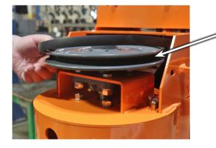
Remove the belt from the motor and driven shaft sheaves as shown in the photo on the left.
