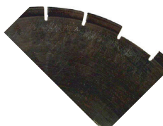
Segment Loss: Usually insufficient water
