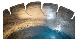
Cracked Segments And or Core Wrong Blade for job
