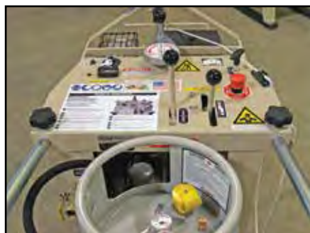
SS-20 Console-Mounted Controls
