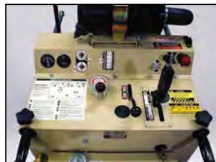
SS-30 Console-Mounted Controls
